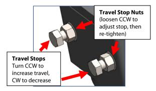
For example, if the valve is not closing all the way, the rotation in the closed direction needs to be increased (to close more). Loosen the CLOSE travel stop nut (on the right), and turn the CLOSE travel stop counter-clockwise (CCW). Manually operate the valve to test the new, adjusted closed position. Once the desired position is reached, tighten the travel stop nut to lock in place.
