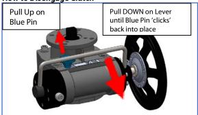
\*Note: For spring return actuators, return actuator to relaxed spring position before disengaging clutch
