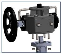
Gear operator is attached to valve by 4 or 8 bolts/studs (body tapped). A female drive is designed to accept a male valve stem or coupling w/ slip fit clearance.
